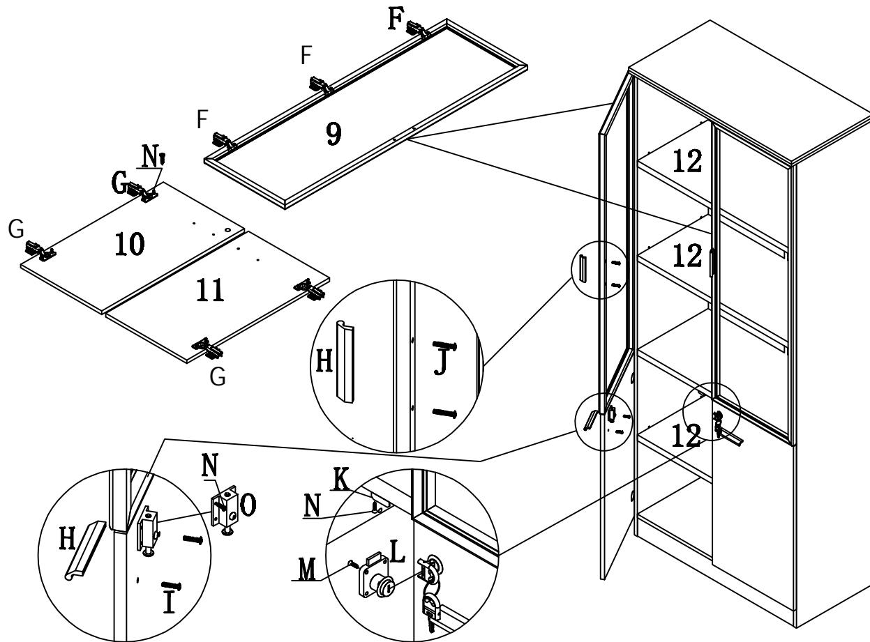
To fix the inside lock O on left wood door and fix the handles for all doors
